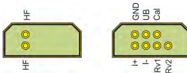
Fig. 5: SV_3a_PCM16, Pin assignment
