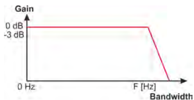
Fig. 6: Gain bandwidth characteristic
